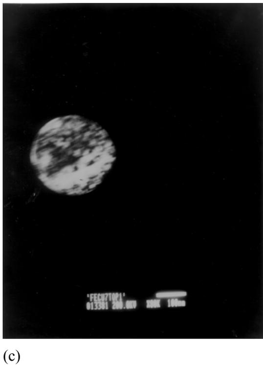
Figure 3.13 Microstructures near the top of the Cu-Fe weld at 5.5 kW, 21 mm/s. (a) bright field image of the bcc-Fe globule (b) Selected Area Diffraction pattern from the globule showing [001] zone of bcc-Fe and (c) dark field image from the  $(\bar{1}\bar{1}0)$  reflection.
