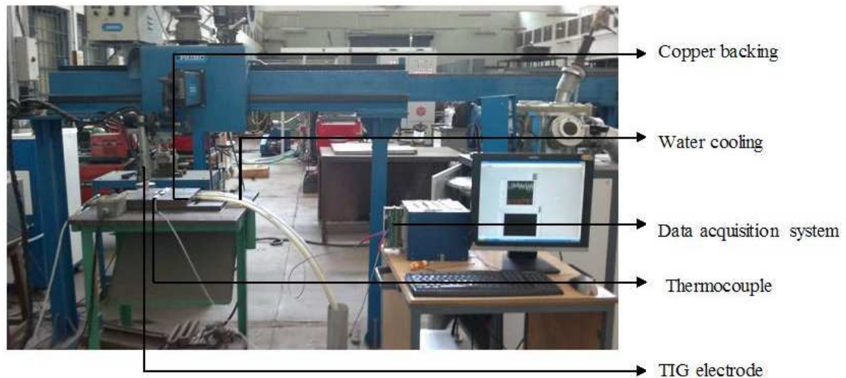
Fig. 1. Typical bead-on plate weld showing copper backing and water cooling arrangements.
