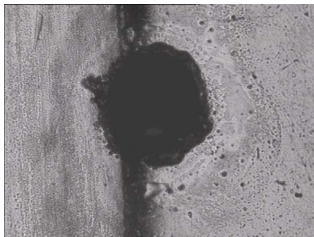
Figure 8b. Top view of a spot weld taken with Nd-YAG laser with a 300 mJ pulse.
