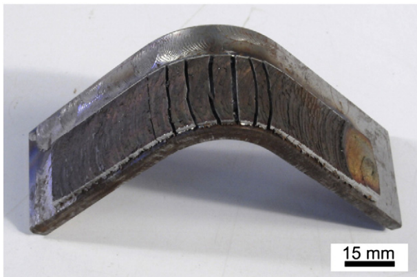
Fig. 18. Close-up picture of a bent coating, produced using a mechtrode rotational speed of 1600 rpm.
