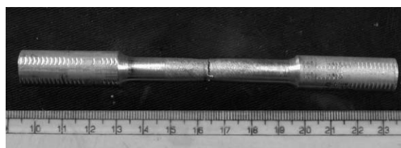
Fig. 2. Fractured weld tensile specimen (Sample S7).
