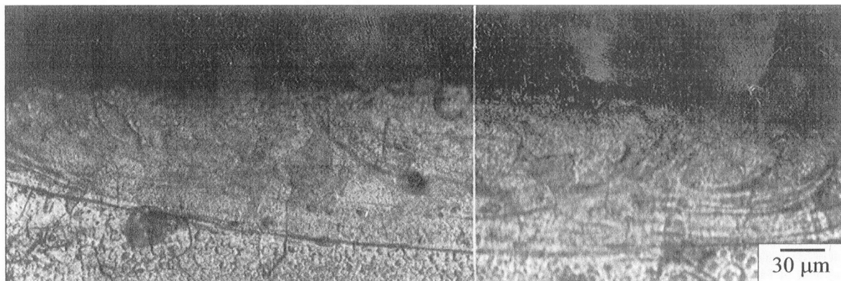
Fig. 1—Optical micrograph revealing the cross-section morphology of the laser-alloyed pool processed at a scan rate of 51 mm/s.
