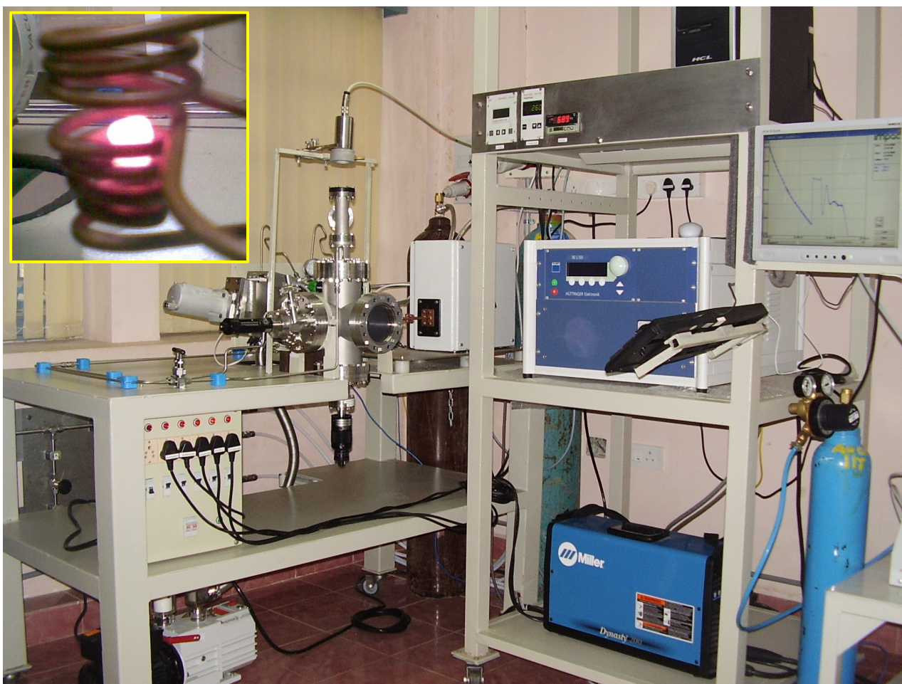
Electromagnetic Levitation Setup for undercooling of metallic melts. Inset shows a levitated nickel droplet.
